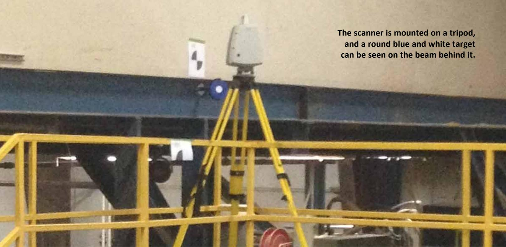
The scanner is mounted on a tripod, and a round blue and white target can be seen on the beam behind it.
